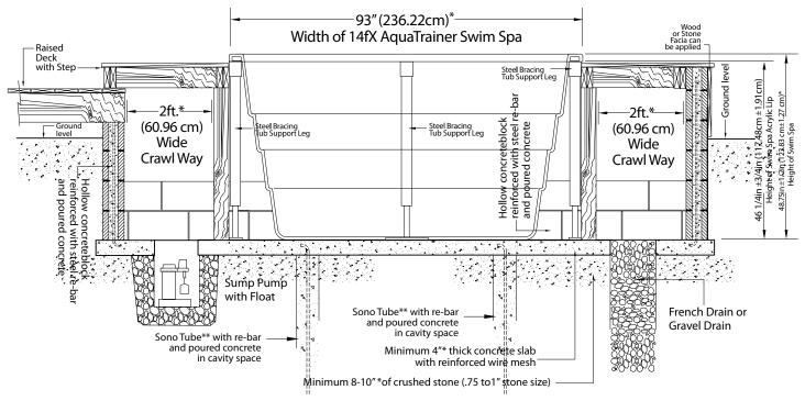
rided as a guide only. As each Swim Spa installation has its own set of chal \*\* Sono Tubes only required in installtions that are in regions that experience freezing and thawing.
